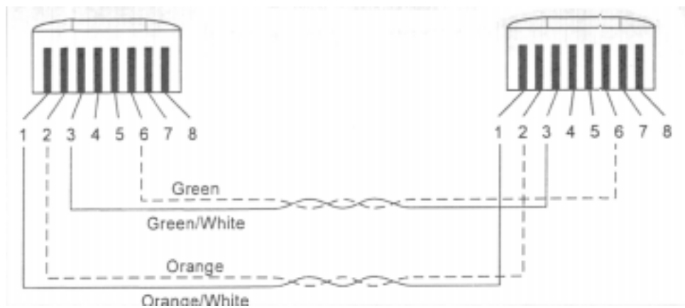
Figure C-2. Straight-Through UTP Cable (RJ-45 to RJ-45), T568B
