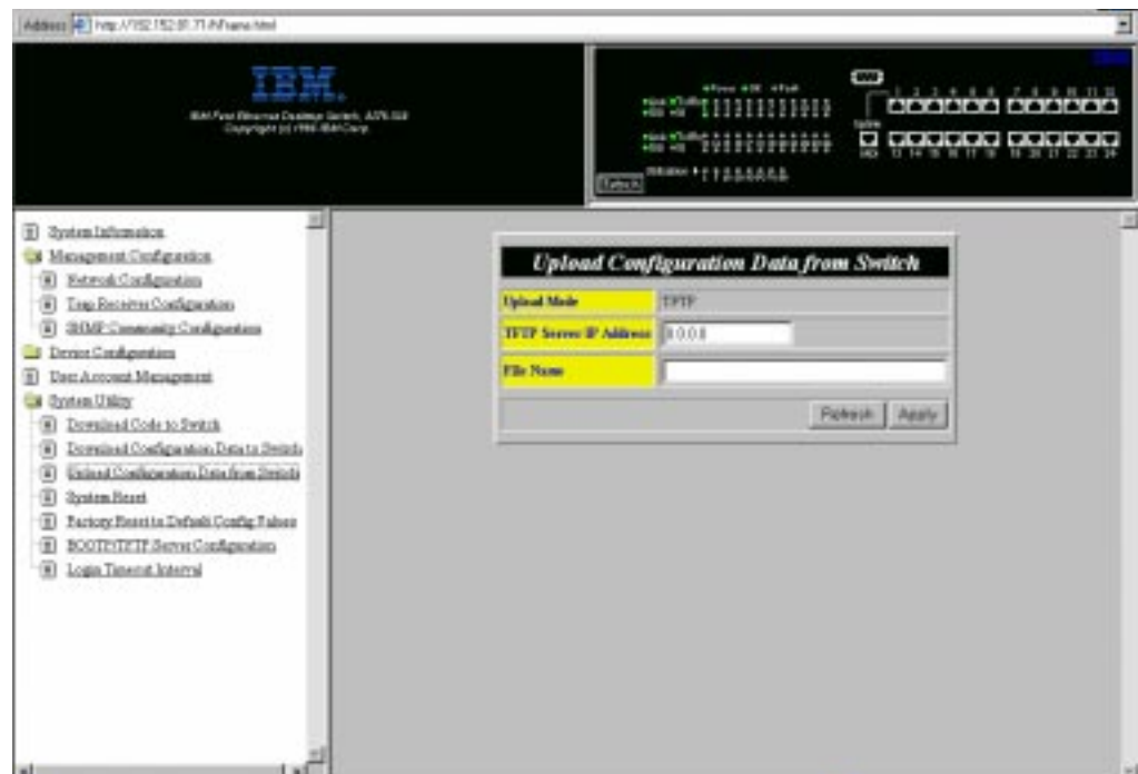
Figure 5-18. Upload Configuration Data from Switch Panel
