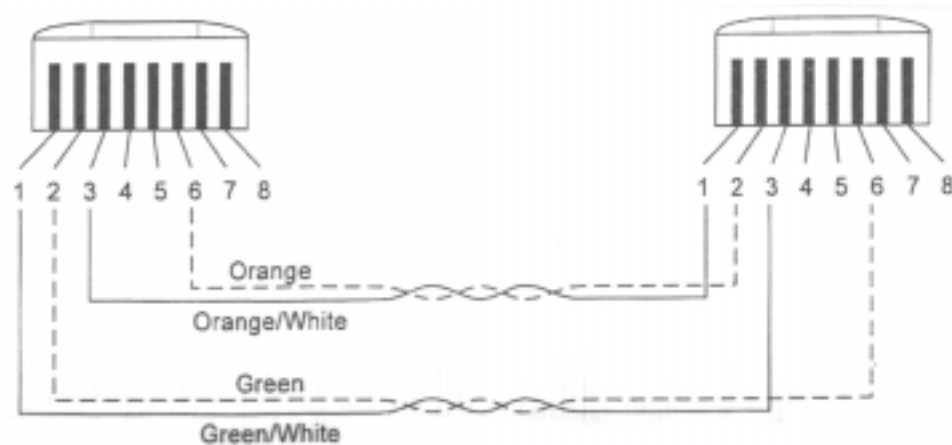
Figure C-4. Crossover UTP Cable (RJ-45 to RJ-45), T568-A
